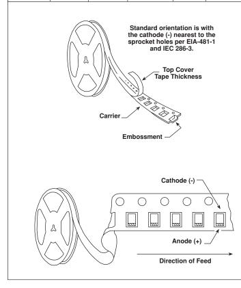
**Tape and Reel Specifications**: All case codes are available on plastic embossed tape per EIA-481-1. Tape reeling per IEC 286-3 is also available. Standard reel diameter is 13" [330mm]. 7" [178mm] reels are available.
